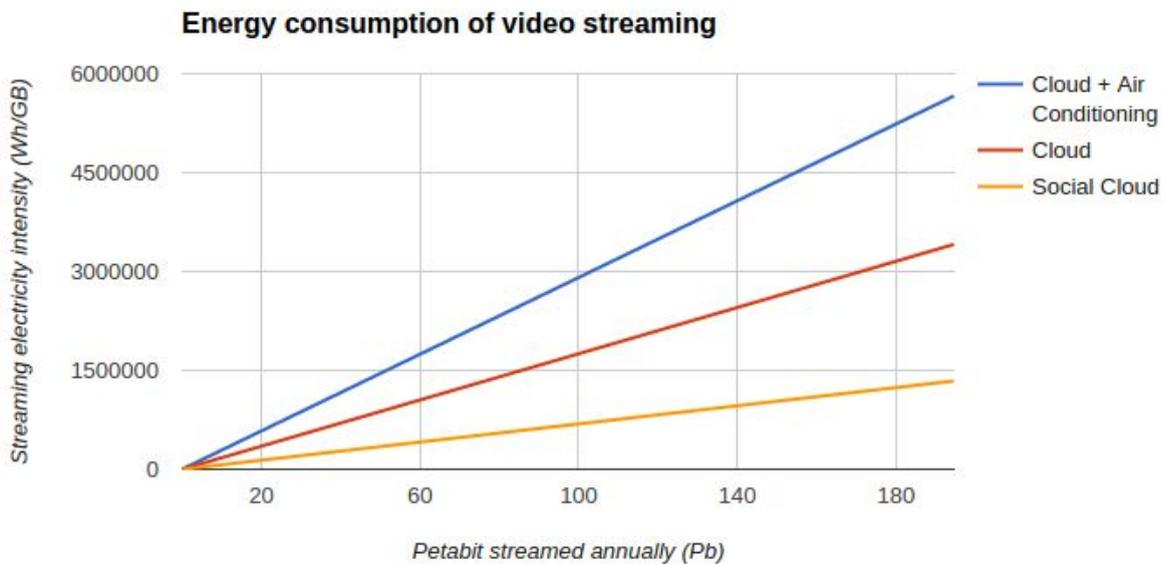
This study is mainly focused on the consumption of the computer resources needed to provide video streaming but the infrastructure used by the datacenters to protect and maintain these resources are worth studying. This figures shows the energy cost of cooling the servers with air conditioning according to a study published in 2014<sup>11</sup>. These results demonstrates that a big quantity of energy is used by servers and can be saved in the social cloud model.
